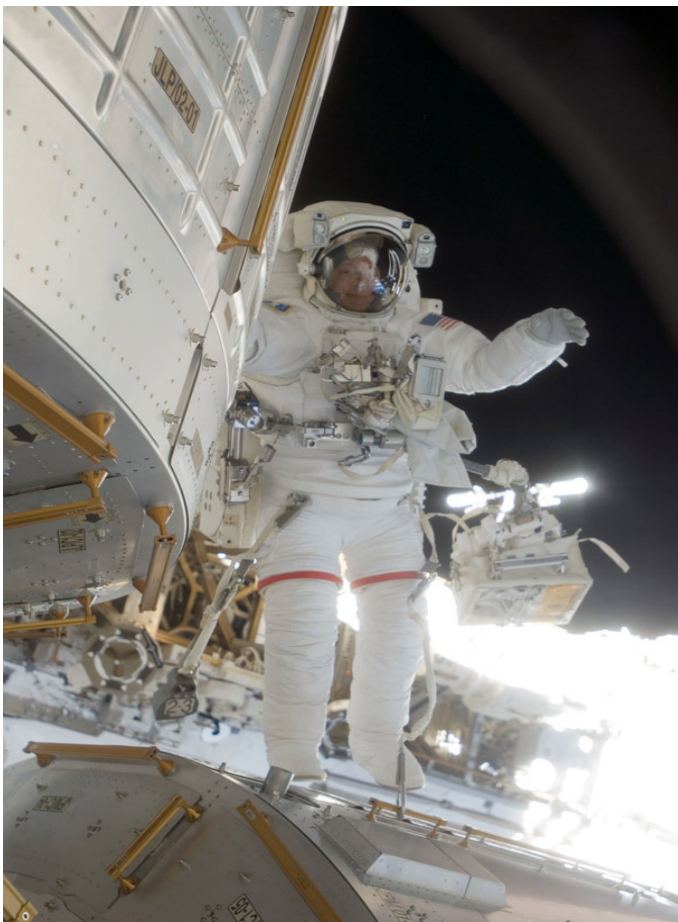
Astronaut Mike Fossum, participating in the mission's second scheduled session of extravehicular activity. During the seven-hour, 11-minute spacewalk, Fossum, installed television cameras on the front and rear of the Kibo Japanese Pressurized Module, removed thermal covers from the Kibo robotic arm and prepared an upper docking port for flight day seven's attachment of the Kibo logistics module. (AP Photo/NASA)
